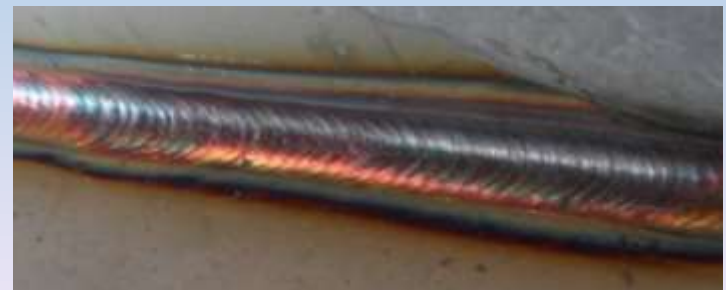
Kehlnaht 12mm VA WIG-Stab 3,2mm
